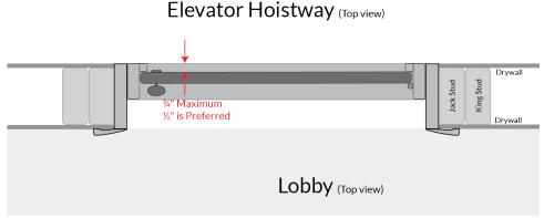
2. The distance between the hoistway face of the landing door or gate must reject a 4" diameter ball at all points. Inability to meet this requirement will create a SAFETY ISSUE and can result in INJURY, DEATH, or a Failed Inspection. See below.
