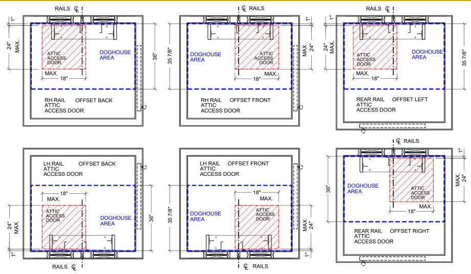
IF ACCESS DOOR IS IN CEILING OF THE ELEVATOR SHAFT, THEN CONTROLLER, VVVF DRIVE, UPS, ELECTRICAL BOXES, GFI, PHONE LINE & LIGHT FIXTURE & SWITCH TO BE LOCATED IN ATTIC.
