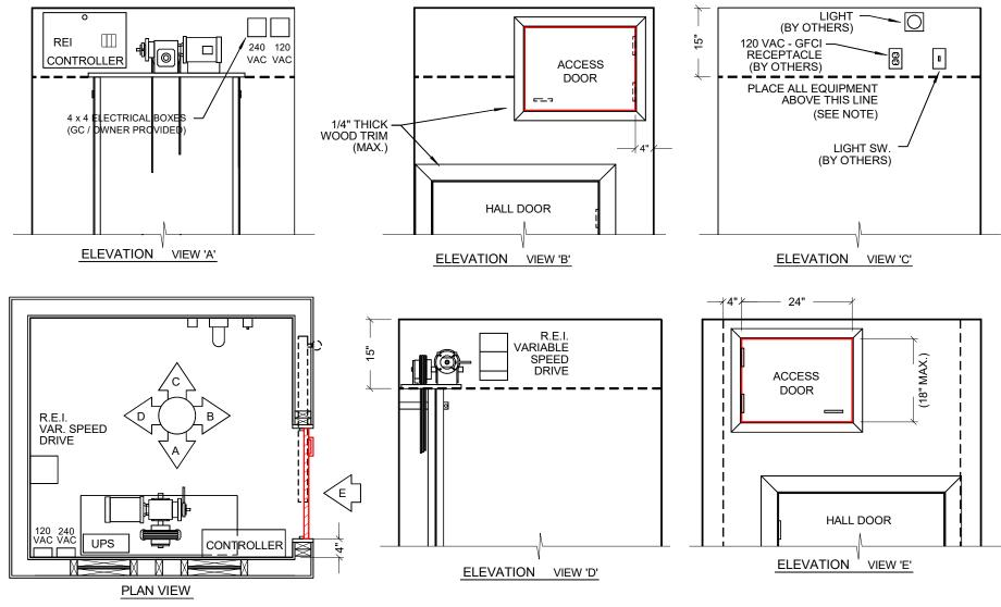
NOTE: LIGHT FIXTURE, LIGHT SWITCH, RECEPTACLE AND ELEC. BOXES CANNOT BE MOUNTED LOWER THAN 15" LINE FROM CEILING.
