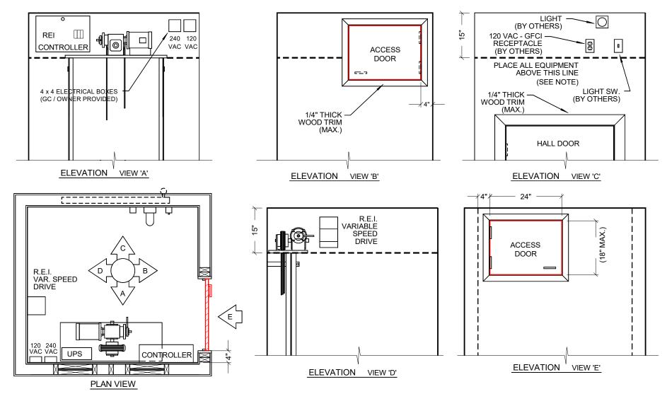
NOTE: LIGHT FIXTURE, LIGHT SWITCH, RECEPTACLE AND ELECTRIC BOXES CANNOT BE MOUNTED LOWER THAN 15" LINE FROM CEILING.
