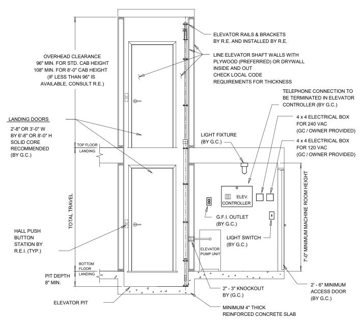
RESIDENTIAL ELEVATORS (RE) CONTROL SYSTEM CONTAINS THE 240 VAC AND 120 VAC DISCONNECTS, HOWEVER; GC / OWNER MUST PROVIDE DEDICATED CIRCUIT AND WIRE TO 4" x 4" BOX (1 FOR 240 VAC & 1 FOR 120 VAC) IN MACHINE SPACE PER DRAWING. SEE RE ELECTRICAL REQUIREMENTS BROCHURE FOR FURTHER DETAILS.
